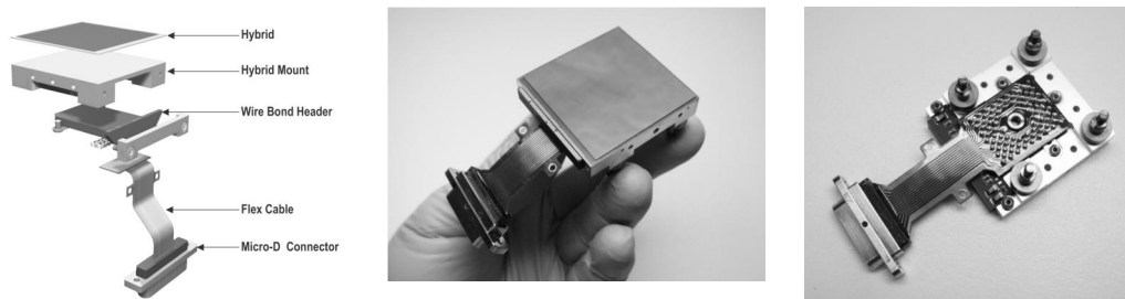
Figure 5. NIRSPEC uses two Rockwell H2RG Sensor Chip Assemblies (SCA's) sensitive over the \lambda = 0.6 - 5 \mu\text{m} wavelength range. From left to right are shown: (1) exploded assembly view of SCA, (2) SCA viewed from top, photo-sensitive side, and (3) SCA viewed from underside. The Hybrid consists of a substrate-removed HgCdTe detector array indium bump-bonded to a H2RG readout integrated circuit (ROIC).
